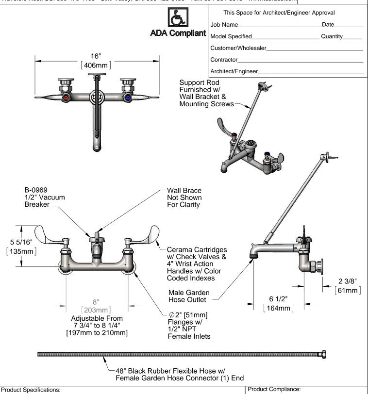
8" Wall Mount Service Sink Mixing Faucet, Cerama Cartridges w/ Check Valves, 4" Wrist Action Handles, 1/2" NPT Vacuum Breaker, Upper Wall Brace, 48" Black Rubber Flexible Hose & 1/2" NPT Female Inlets
